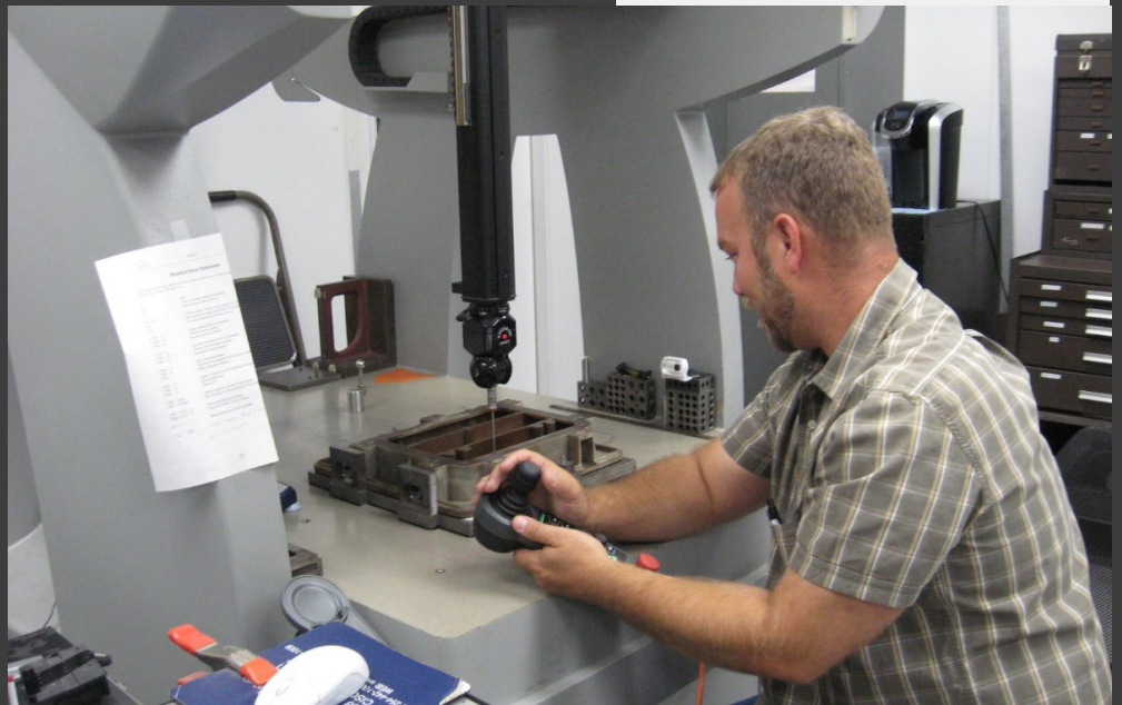
Quality Manager Daniel Bray is shown here inspecting a part on the CMM.
